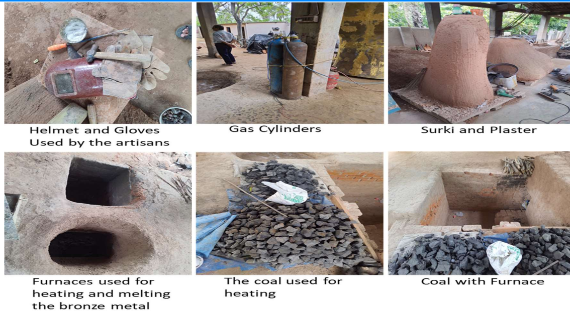
Figure 3: Infrastructure and equipment used for bronze casting.
